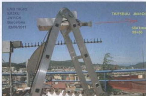
EA3XU, JN11CK, wkg TK/F5BUU on 10 GHz over 584km with just a horn
