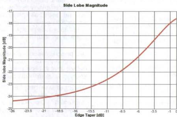
Fig. 1 – The level of the first sidelobe as a function of the edge taper for quadratic distribution.
