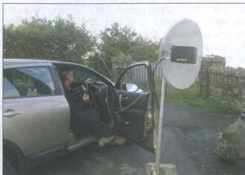
Photo 1: A picture from the Knockagh Monument during G1CET/P and G1GATZ/P (Sieve Croob) contact on 3cm SSB and DB6NT transverter 200mW into vertical Sky dish, excellent signals. Photo G10GDP
