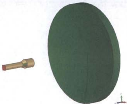
Fig. 5 – Prime focus dish antenna configuration
