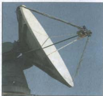
Fig. 2: 4,5m dish at OK1KIR for 3,4 GHz (from G3LTF present.)
