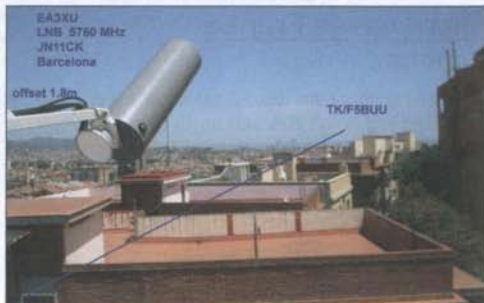
EA3XU, JN11CK, wkg TK/F5BUU with 5.7 GHz LNB setup
